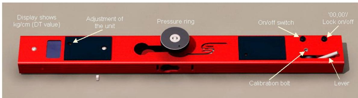
The picture shows the functions of the Stringlab 2 measuring system:
