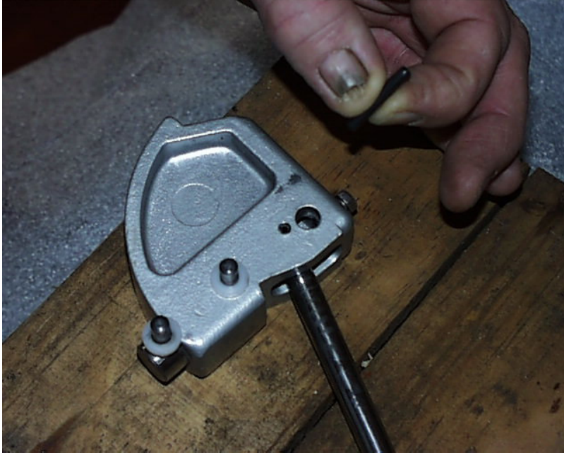
Fig. 10 Replacing the pin.
