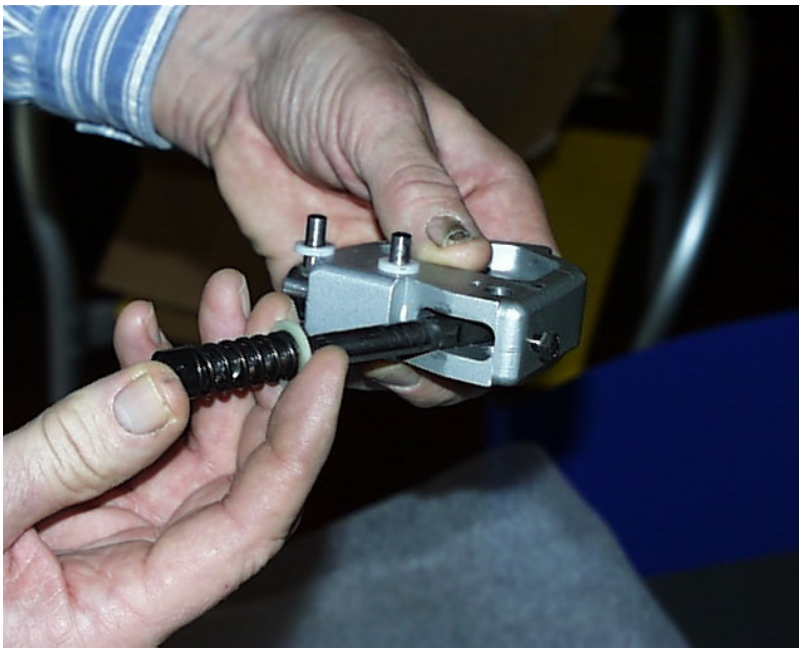
Fig. 9 Take the upper bush, the spring and the washer of the pullrod.
