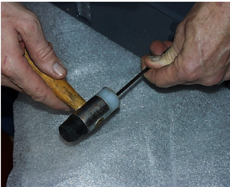
Fig. 3 If necessary use a plastic hammer to push the pin out gently.
