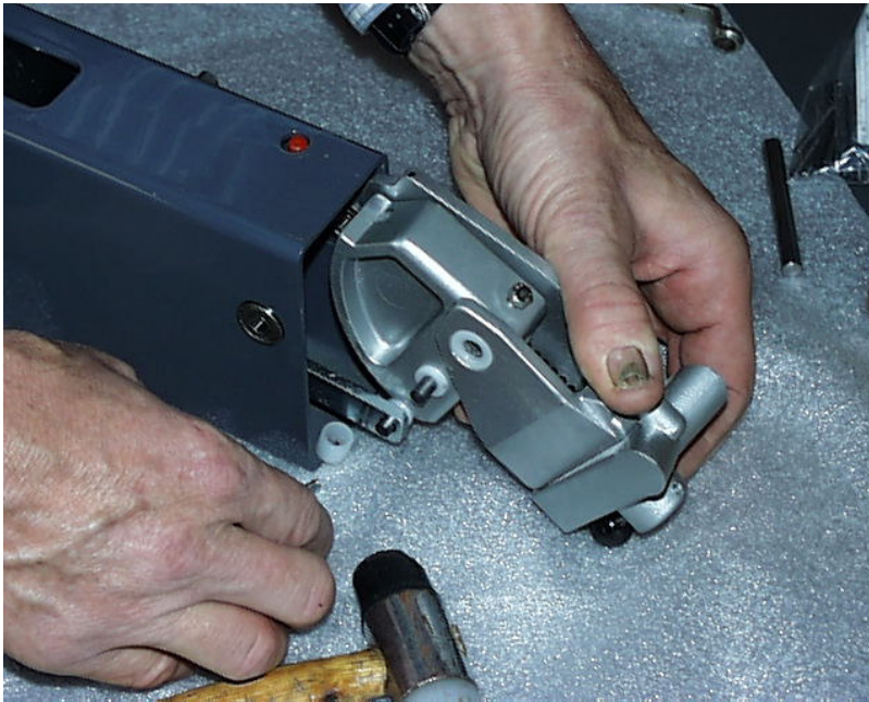
Fig. 4 Take the tension head out of the housing.
