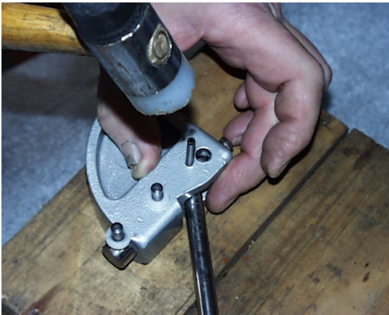
Fig. 11 Hammer the new pin into the hole and at the same time the old pin out.
